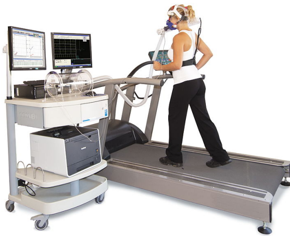
Metabolic Cart is Used to Measure Energy Expenditure in Exercise Settings
